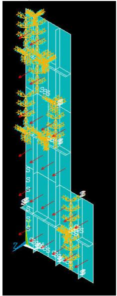
We see that the symmetry and clamped BC's haven't been applied at the correct locations. The pressure has been applied only over part of the facesheet. We'll fix these mistakes below.
