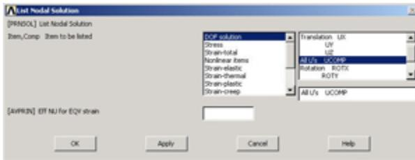
From the list, the displacement amplitude, denoted as **USUM**, is 23.9e-3. The corresponding value in table 11.17-1 is 23.8e-3. Similarly, you can determine the other entries in the table. Note that the rotational d.o.f. to use for the second row in the table is **ROTZ**...—
