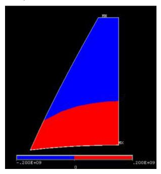
The FEA results indicate that the neutral axis is curved, contrary to the assumption in mechanics of materials theory.
