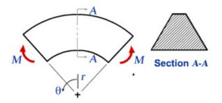
We would like to obtain the stresses for the trapezoidal cross-section AA shown above. Stresses in the curved beam do not vary with , so we can reduce the model and analyze only a typical slice between two closely spaced radial planes as shown below. The angle between AB and CD is taken to be 5 deg. as suggested by Cook et al.
