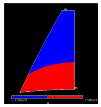
The FEA results indicate that the neutral axis is curved, contrary to the assumption in mechanics of materials theory.
