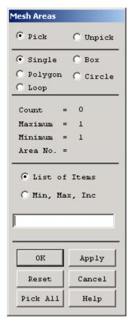
In the *Input* window, ANSYS tells you to "pick or enter areas to be meshed". Since we have only one area to be meshed, click on *Pick All*. The geometry has been meshed and the elements are plotted in the *Graphics* window. *Close* the *MeshTool*.
