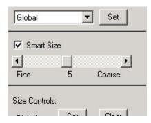
The only input necessary for the *SmartSize* option is the overall element size level for meshing. The element size level determines the fineness of the mesh. Its value is controlled by the slider shown in the above picture. Change the setting for the overall element size level to 5 by moving the slider under *S martSize* to the left.
