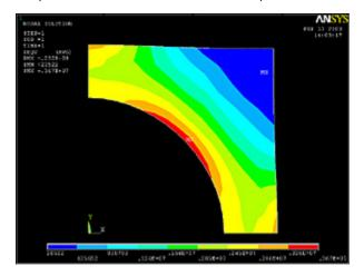
The two results compare well with the finer mesh contours being smoother as expected. Compare the maximum stress and displacement values:
