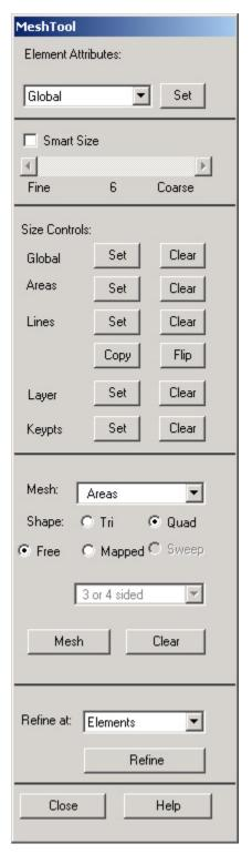
This brings up the Meshing Attributes menu. You will see that the correct element type and material number are already selected since we have only one of each. Recall that no real constants need to be defined for PLANE42 element type with the plane stress keyoption.
