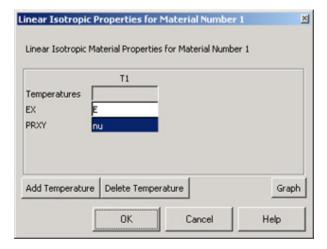
To double-check the material property values, double-click on *Linear, Isotropic* under *Material Model Number 1* in the *Define Material Model Behavior* menu. This will show you the current values for *EX* and *PRXY*. *Cancel* the *Linear Isotropic Properties* window.
