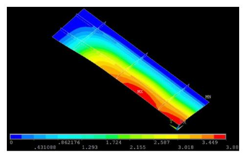
The location of maximum deflection  $w_{max}$  is labeled MX. This occurs not at the facesheet center but on the edge x=0, at approximately y=L1/3. As expected, the deflection is zero along the clamped edges.
