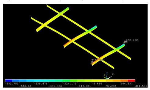
The  $_{xx}$  values for the stiffeners in the y-direction is virtually zero; confirm this using **Query Results**. This means that, as expected, the load in the x-direction is carried by the stiffeners in that direction.
