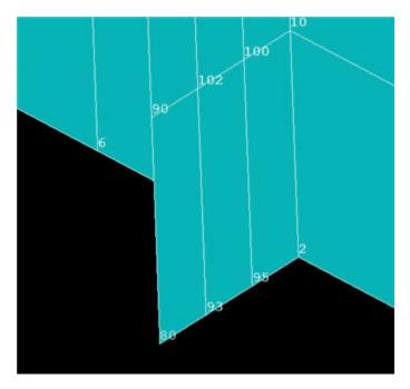
If you performed the merge operation correctly, you'll see that the higher numbered node has been deleted and the two coincident nodes have been replaced by a single node.
