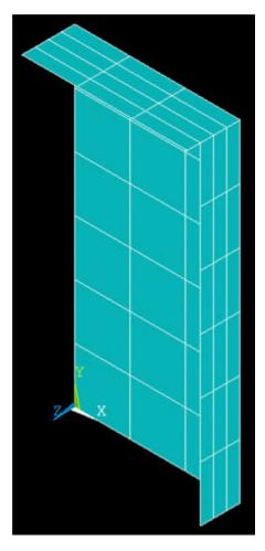
Let's change the graphical display so that the geometry is displayed as a solid model with the shell thicknesses shown. At the command prompt, type /esh ape, 1 and then select **Utility Menu > Plot > Replot**. When the /ESHAPE command in issued, ANSYS uses the real constants associated with each element to determine its shape. (Note that commands are not case-senstive.)
