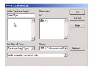
Search for the *plate2.lwg* file in the directory you specified and open it using notepad. Then save this file as *plate2.txt*. This is the log/input file we will modify. The list of commands generated is shown below.
