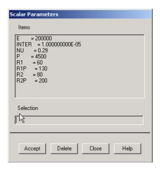
Close the Scalar Parameters window. Note that we have specified the radii in mm, the load p in N and the Young's modulus in N/mm<sup>2</sup>. Therefore, the displacement results we obtain will be in mm and the stresses in N/mm<sup>2</sup>.
