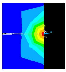
The contour plot also shows the locations of the maximum and minimum values with the labels MX and MN, respectively. As you can see, the upper and lower disks have deformed and come into contact.
