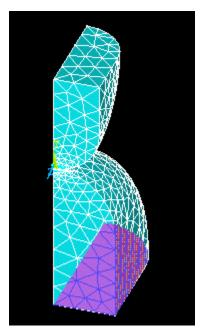
This brings up the Apply U,Rot on Areas menu. Select UY for the DOFs to be constrained and enter 0 for the Displacement value. Click OK.
