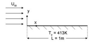
In our problem, we have a flat plate at a constant temperature of 413K. The plate is infinitely wide. The velocity profile of the fluid is uniform at the point x = 0. The free stream temperature of the fluid is 353K. The assumption of incompressible flow becomes invalid increasingly less valid for larger temperature differences between the plate and freestream. Because of this, we will treat this as a compressible flow. We will analyze a fluid flow with the following non-dimensional conditions:
