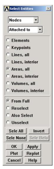
Check that only nodes attached to face 1 are currently selected: Utility Menu > Plot > Nodes
