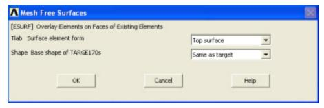
This brings up the Mesh free Surfaces pick menu. In the Input window, ANSYS tells you to "pick or enter node for contact elements". Since we have already selected the nodes, click Pick All.
