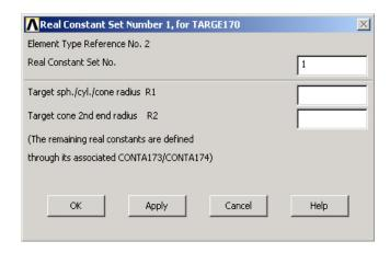
Real constants R1 and R2 define the geometry of the target elements. For contact problems, it is recommended to first try using the default settings, and then change them if difficulties are encountered or the analysis has special situations. ANSYS will default R1 and R2 to zero once the target elements are generated. We'll use the default values for our analysis. Click *Cancel*.
