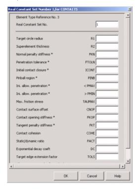
As you can see, ANSYS uses several real constants to control contact behavior. As in the previous case, we'll use the default values set by ANSYS for our analysis. Refer to the help page for *CONTA175*, for a detailed description of the real constants for this element.
