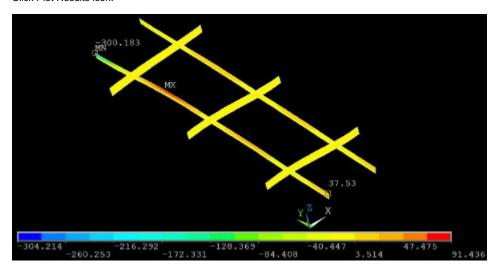
The yy values for the stiffeners in the x-direction is virtually zero; confirm this using **Query Results**. This means that, as expected, the load in the y-direction is carried by the stiffeners in that direction.
