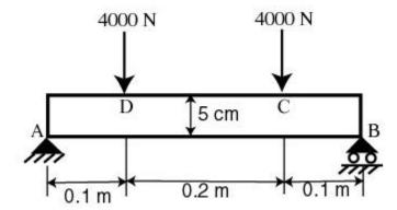
An alternative scenario is that we get clever and force *C* and *D* to be corner points. This can be done by dividing the geometry into three rectangles *R1*, *R2* and *R3*as shown below. This will force nodes to be created at points C and D. Then, the point forces can be applied to these nodes. This is the strategy we'll use in creating the mesh.
