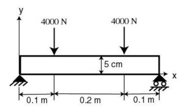
We'll put redAnTS to work on solving this problem using FEA. We'll plot displacements and stresses for the beam and make comparisons with theory.
