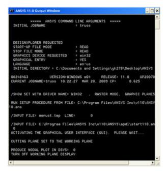
This is the window to which output from ANSYS commands is written and which provides feedback on the actions taken by ANSYS as you navigate the menus. If, at some point, you are not sure you clicked the right button or entered a value correctly, this is where to look first to figure out what you just did.
