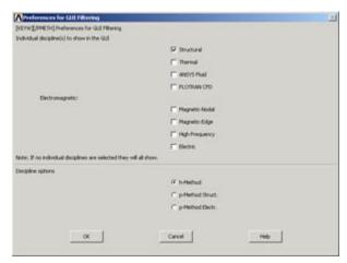
The effect of selecting the structural preference is that only menu options applicable to structural mechanics are shown in the graphical user interface; options related to other disciplines such as thermal, fluid and electromagnetics are grayed out. This helps a little while navigating the vast menu options within ANSYS.
