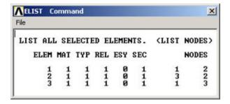
This table says that *Element 1* is of *material type 1* and *element type 1* and is attached to nodes 1 and 2 and so on. In this element list, the order of the two nodes for each element doesn't matter. For example, element 3 can be attached to nodes 2 and 3 or equivalently, nodes 3 and 2. Also, the order of element numbering is not important since it is for internal bookkeeping.
