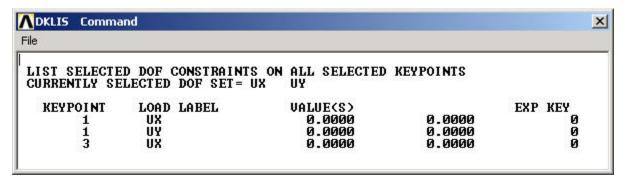
If you made a mistake in applying a constraint, you can delete and reapply it. You can delete a constraint using Main Menu > Preprocessor > Loads > Define Loads > Delete > Structural > Displacement > On Keypoints. Alternately, you can resume from your last save and continue from there.
