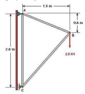
You can see from the diagram that the pin at A is constrained in x and y directions; or equivalently, keypoint 1 is constrained such that its *UX* and *UY* displacements are zero. Similarly, keypoint 3 is constrained such that its *UX* displacement is zero.
