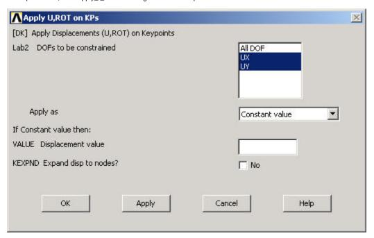
Since we want to constrain *UX* as well as *UY* to zero at keypoint 1, select both UX and UY from items in DOFs to be constrained list. Since the Displacement value is zero by default, leave that field empty. Click on Apply.
