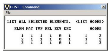
This table says that *Element 1* is of *material type 1* and *element type 1* and is attached to nodes 1 and 2 and so on. In this element list, the order of the two nodes for each element doesn't matter. For example, element 3 can be attached to nodes 2 and 3 or equivalently, nodes 3 and 2. Also, the order of element numbering is not important since it is for internal bookkeeping.
