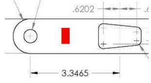
In the coordinate system in our model, let's say this area is given by -1.77" x -1.57" and 0.45" y 0.85". To find the average strain in this area, we will select all nodes that lie in this area and then list the strain values at these nodes. You can copy these values over to Excel or MATLAB to find the average value.
