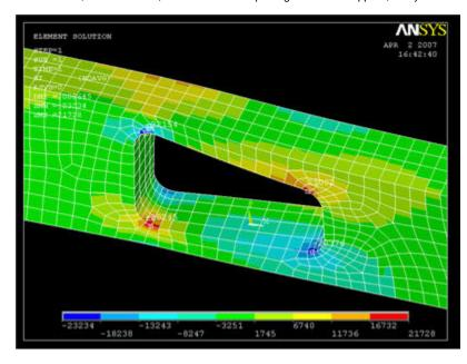
Compare the stress values with the von Mises stress. (Click on von Mises stress, then OK)
