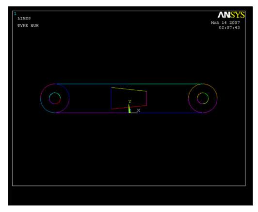
Next, we want to fillet the corners, as specified in the drawing. You can zoom in and out by using the mouse wheel or clicking on the appropriate buttons on the right toolbar (magnifying glass with + or -).
