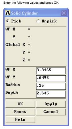
We must now glue the shaft to the crank. The reason for using "glue" instead of performing a boolean add on the volumes is to maintain two discrete parts. This provides more flexibility in modeling, as it can allow for different materials and meshes. Note: If glue is not used, the two pieces will be independent of each other and the solution will be incorrect.
