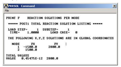
The sum of the reaction forces balances the applied load as should be the case for static equilibrium.
