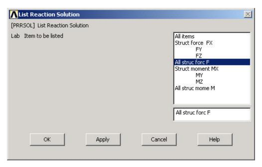
This brings up a window with the reaction forces at the nodes.
