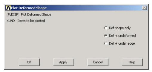
This plots the deformed and undeformed shapes in the Graphics window.
