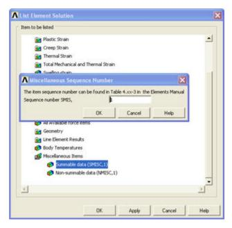
This brings up a window with the axial forces in the elements. Positive values indicate tension and negative values compression. Do these values match what we got in method 1?
