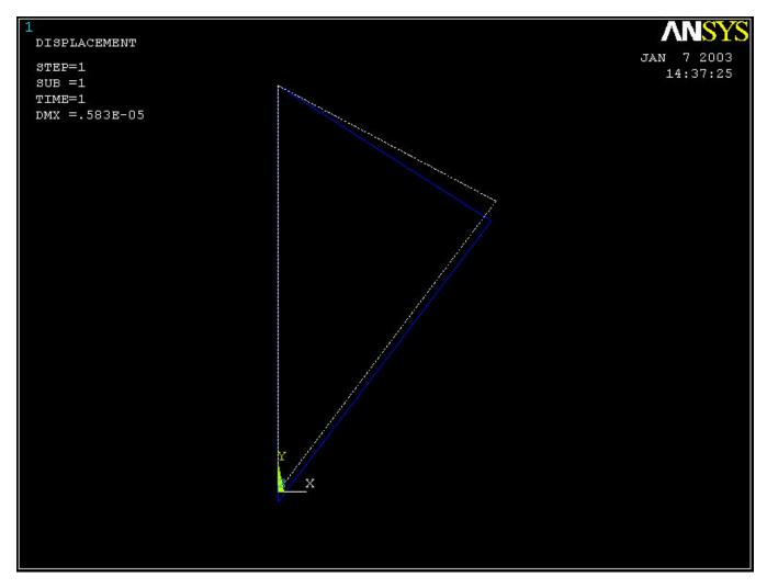
The deformed shape is shown as a solid line and the undeformed shape as a dotted line. The maximum displacement *DMX* is 0.583E-05m as reported in the *Graphics* window. This is small but plausible. Note that the deformation is magnified in the plot so as to be easily visible.
