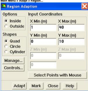
Enter 1 and 40 for X Min and X Max. Enter 0 and 10 for Y Min and Y Max. Click Mark. FLUENT will print the following message in the console window: 5416 cells marked for refinement, 0 cells marked for coarsening
