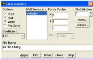
Under Coefficient, select Lift. Select cylinder under Wall Zones. Under Options, select Print, Plot and Write. Note that Plot Window is 1. Click Apply.
