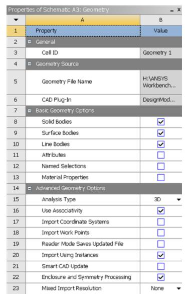
In the *Project Schematic*, double left click on *Geometry* to start preparing the geometry.
