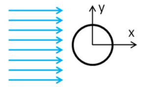
Consider the unsteady state case of a fluid flowing past a cylinder, as illustrated above. For this tutorial we will use a Reynolds Number of 120. In order to simplify the computation, the diameter of the cylinder is set to 1 m, the x component of the velocity is set to 1 m/s and the density of the fluid is set to 1 kg /m^3. Thus, the dynamic viscosity must be set to 8.333x10^-3 kg/m\*s in order to obtain the desired Reynolds number.
