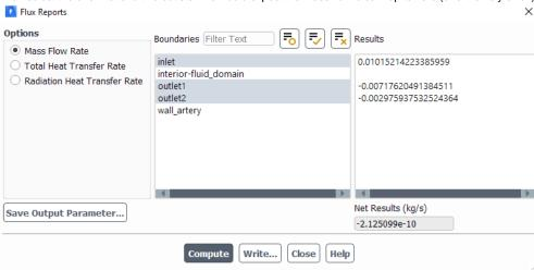
As we can see from the window above, the mass fluxes add up to -2.125e-10, which is very close to zero. Thus, we can conclude that mass is conserved in the simulation.
