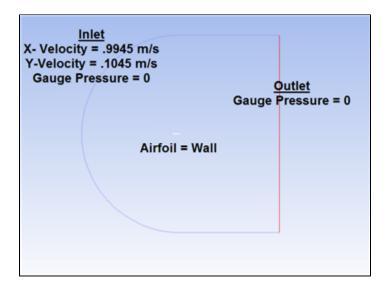
The edges highlighted blue are the inlet, the edges highlighted red are the outlet, and the airfoil is highlighted white in the middle. Now we are ready to
