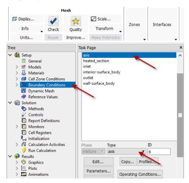
Now let's specify the boundary condition at the walls. By default, FLUENT correctly picks the Wall boundary type for these boundaries. It will impose the no-slip condition for velocity at these boundaries. Additionally, for the heated wall section, we need to specify the heat flux into the flow.
