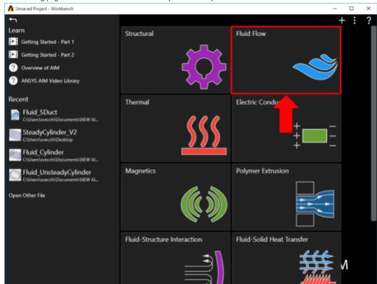
You will be prompted by the Fluid Flow template to either Define new geometry, Import geometry file, or Connect to active CAD session. Select Import geometry and press Next.
