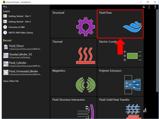
You will be prompted by the FI uid Flow template to either Define new geometry, Import geometry file, or Connect to active CAD session. Select Define new geometry and press N ext. Finally, check the Swirling flow box in the Additional flow physics and press Finish.
