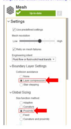
AIM will prompt you to fix the boundary layer before generating the mesh. Click on **Boundary Layer** under **Mesh Controls**. Select every face except for the circular inlet and outlet faces. An easy way to do this is drag a square around the shape and then deselect the inlet and outlet using CTRL + click.
