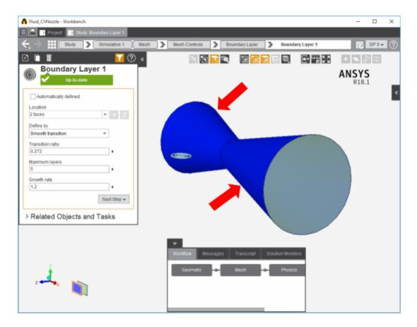
We will also change the mesh to use hexahedrons, to more accurately capture the effects in the critical nozzle region and aid convergence of the calculations. Click on **Mesh Controls**, then **Element Shape 1**. Change the **Shape** to **Hexahedrons**.
