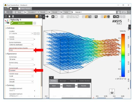
To find the total pressure on the walls of the duct, return to the **Results** task and select **Contour** from the **Add** dropdown menu. Select all of the outside faces of the flow volume (except the inlet and outlet) and change the **Variable** to **Total Pressure**. This will plot the pressure on the duct walls.
