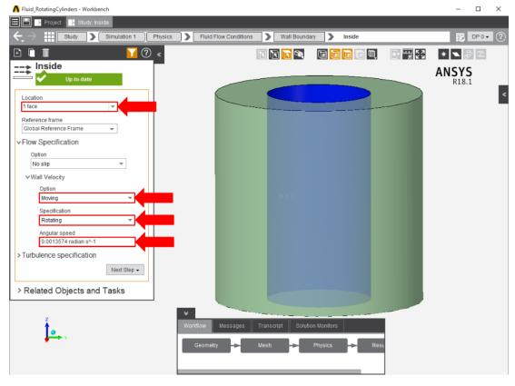
Now that the wall boundary has been created for the inner flow volume face, making the wall boundary for the outer flow volume face will be similar. Select the outer face of the enclosure and select **Wall** from the **Add** drop down menu.
