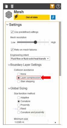
AIM will prompt you to fix the **Boundary Layer** before generating the mesh. Click on **Boundary Layer** under **Mesh Controls**. Select every face except for the inlet and outlet faces (133 faces total).
