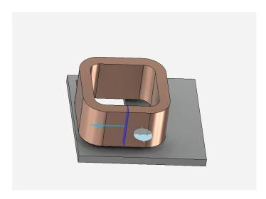
Input an **Operating Current** of 2.742 Amps and 1000 for **Number of Conductors**.
