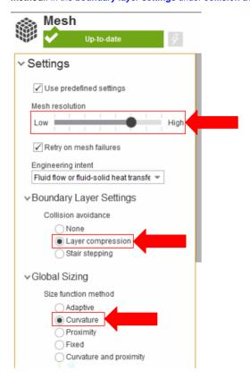
AIM will prompt the user to fix the boundary layer before generating the mesh, click on **boundary layer** under **Mesh Controls**. Select every face except for the future inlet and outlet faces.
