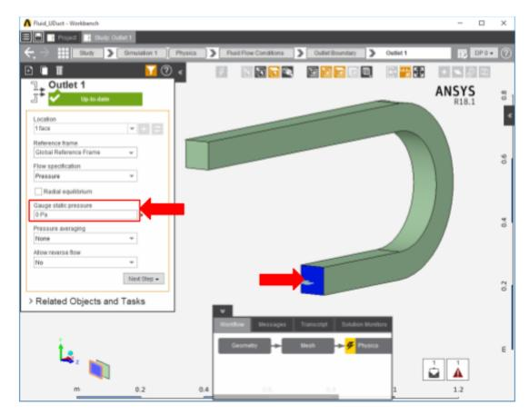
Next a wall condition must be added to all surfaces that are not already defined. Wall can be found in the same Add menu as the previous conditions. AIM will automatically create the walls once the option is selected, AIM selects every face that doesn't already have a constraint on it.
