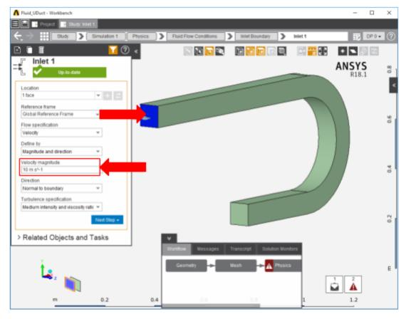
Once the inlet is defined, the outlet is next. In the same menu, use the outlet tool to define an outlet at the small end of the duct. Assign a **Gauge Static Pressure** of 0 psi.
