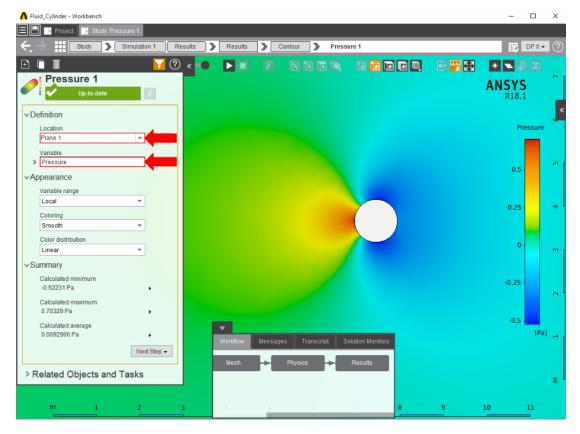
To find the total pressure on the walls of the flow volume, add another **Contour**, select the face of the flow volume in contact with the cylinder, and change the **Variable** to **Total Pressure**.
