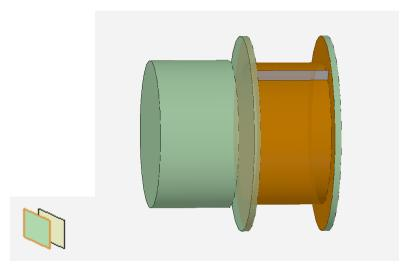
Select the surface by looking for the line in the line that runs perpendicular to the spool face. Click on the plane below the line by using the plane selector. Then input a **Current** of .01 amps and 280 for the **Number of Conductors**. Click on the arrow below to parameterize the **Operating Current**.
