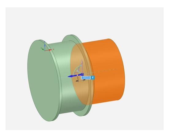
To create the parameter, click on the  $\bf P$  next to the highlighted dimension box. Once the parameter is created, click the x in the top right corner to begin the physics set up.
