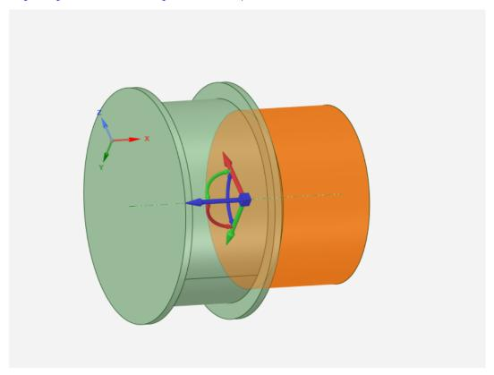
Once the origin turns into a square, select the blue axis of the **Move** tool. The other axis will be greyed out and in the **General** sidebar select the **Ruler** tool. The **Ruler** tool will then follow the cursor, at which point click the face of the spool closest to the inside the gap.
