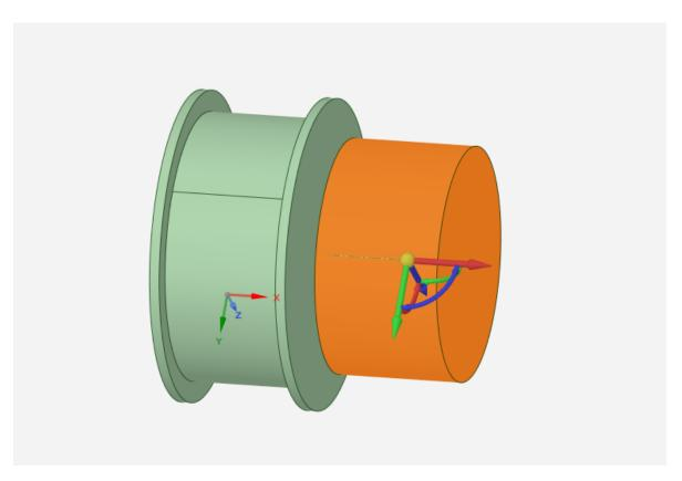
Drag the origin onto the face of the magnet closest to the spool.
