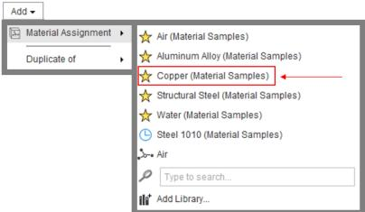
Then click on next step and repeat the process, assigning **Steel 1010 (Material Assignment)** to the yoke and center pole by control selecting both and click on the "+". (You can use "Type to Search" to find **Steel 1010** in the material library.)
