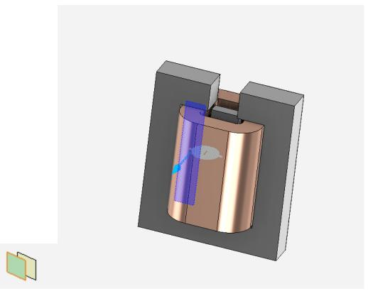
Click the "+" next to cross-sectional face or body. Input 5 A for the Operating Current and 200 for the Number of Conductors.
