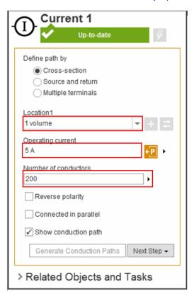
Click on the small arrow next to the operating current box. Select the P to parametrise current. Then click on Generate Conduction Paths, this will show the solver interpretation of the coil. If the solver's interpretation of the coil is incorrect (current is flowing outside of the coil) insulating boundary conditions must be added to ensure that the current stays within the coil. For this model an insulating condition is not required.
