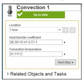
No boundary conditions are required on the symmetry surfaces as a symmetry boundary condition for electric conduction and heat transfer is a natural (unspecified) boundary condition. Now that the Boundary conditions are set, the results are ready to be calculated.
