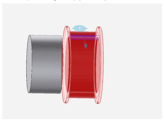
Right click > Add > Electromagnetic Conditions > Insulating. Click on the three inside faces of the brass spool. Hiding the coil geometry will make this step easier.
