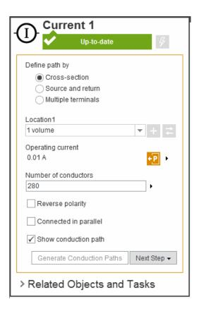
Then click on **Generate Conduction Paths**, this will show the solver interpretation of the coil. If the solver's interpretation of the coil is incorrect (current is flowing outside of the coil) insulating boundary conditions must be added to ensure that the current stays within the coil. Since the solvers interpretation of the coil is incorrect (current is also flowing in the brass spool), insulated boundary conditions will be added.
