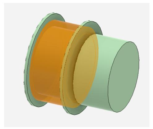
Then, click on next step and repeat the process. Assign NdFe30 (Material Samples) to the magnet and Brass (Material Samples) to the spool. (You can use "Type to Search" to find NdFe30 and Brass in the material library.)
