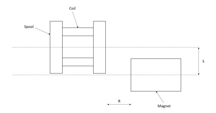
In the first case, the current will vary from from 0-100mA in 10mA intervals. In case two, the axial displacement will vary from 0.0-.5mm in 0.05mm intervals.
