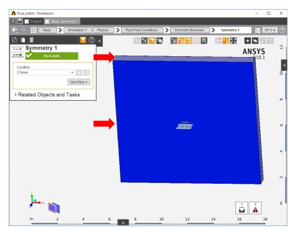
Next, a **Wall** condition must be added to all surfaces that are not already defined. **Wall** can be found in the same **Add** menu as the previous conditions. Mo st of the time, AIM will automatically create the walls once the option is selected; AIM selects every face that doesn't already have a constraint on it.
