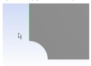
Now look to the Details View window and select *Geometry > Apply*. This should create a red line with a tag on the model. Ensure that under *Symmetry Normal* the x-axis is selected. Repeat this process to create a symmetry region for the bottom edge to the right of the hole, but this time making sure that the *Symmetry Normal* parameter is the y-axis.
